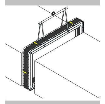
any protective cover and / or shipping straps must **not** be removed until installation is completed, but **must** be removed immediately prior to plant start up
