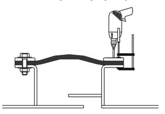
NB It is <u>very important</u> that the clamps (on both sides of the hole) hold the material securely otherwise the fabric and the insulating materials may rotate with the drill, resulting in tearing.
